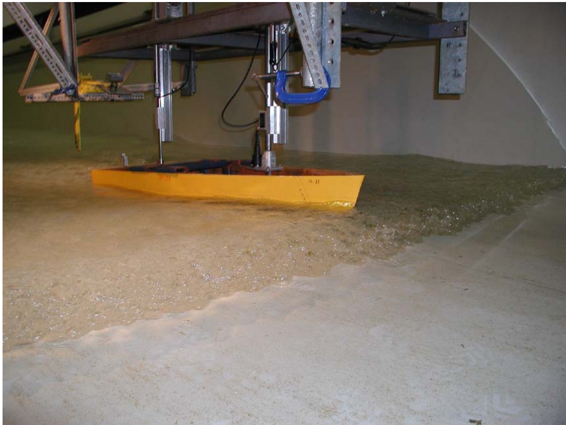
Fig. 2: Free-to-squat model at F_h = 1.35 , showing carriage setup and bore radiating ahead of the model
