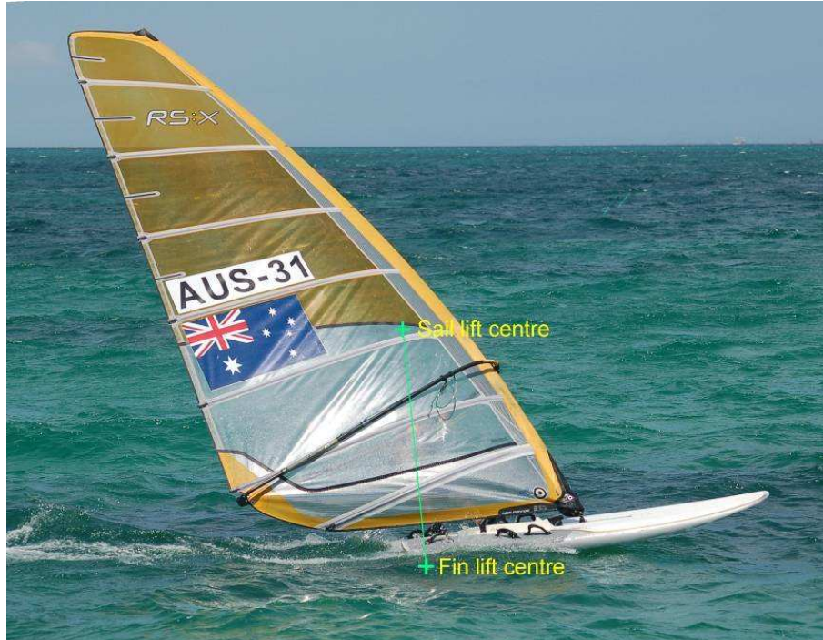
Figure 7: Yaw balance while planing upwind - sail and fin lift centres at similar longitudinal position
