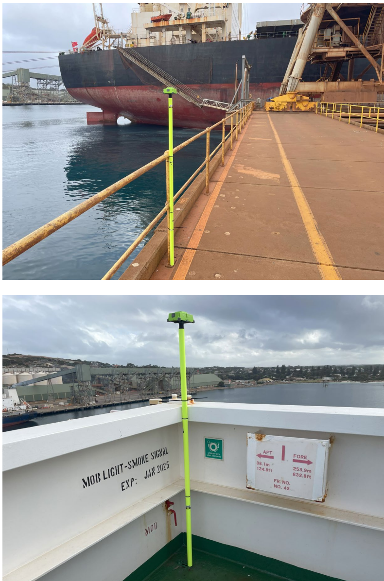
Figure 1: (Top) Fixed base station on Berth 3 jetty; (Bottom) Roving receiver on port bridge wing.
